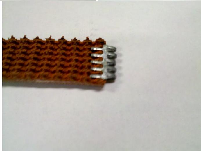
Do the same thing to the other end of the tread, wrap it around your wheel, and slide the pin between the clips. (If you are doing this on a placation wheel, you will need to loosen the wheel to get the tread to fit, after you do this step be sure to tighten the wheel halves together)
