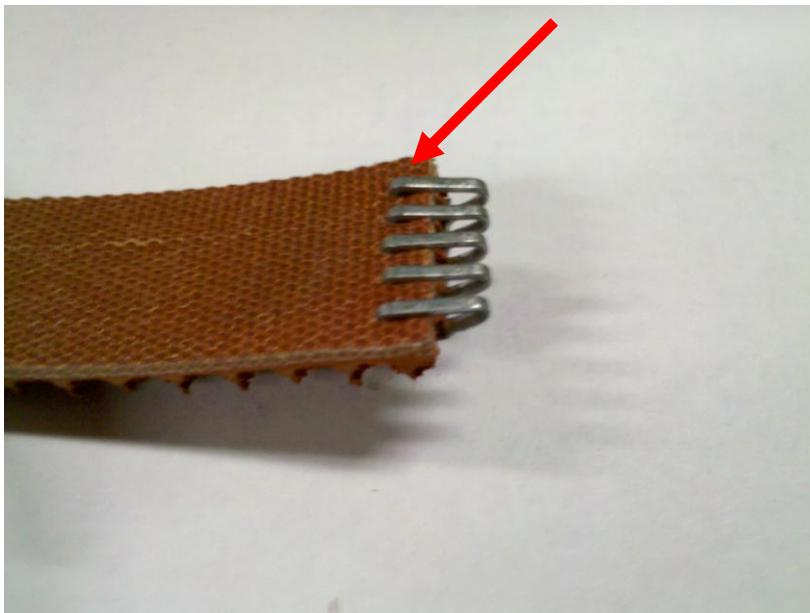
Now flip the tread back over so the tread is exposed, and finish tapping the Alligator Clip tight.
