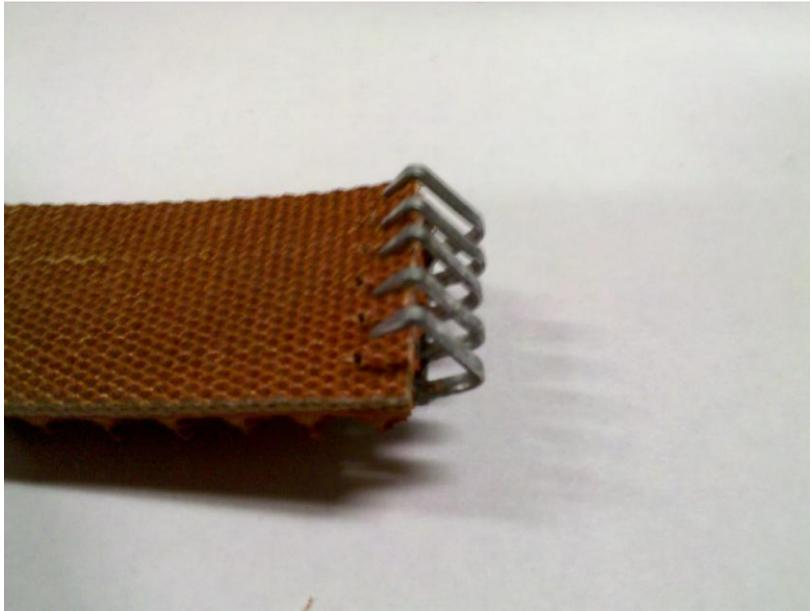
Use a hammer to tap down the longer points into the tread, use a motion more inline with the points.
